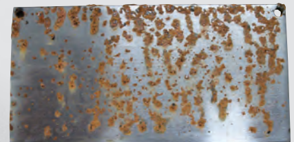
After 192 hours in a humidity cabinet, the metal coupon treated with a leading competitive product rusted severely.
