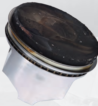
The piston crown contains normal carbon, while the rings remain clean and functional. Note the absence of wear or scuffing on the piston skirt.
