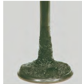
Picture D - Intake valve before P.i. treatment
