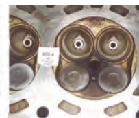
Combustion chamber after P.i. treatment.
